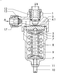
Fig. 4: Type 2357-2 Excess Pressure Valve (PN 50)
