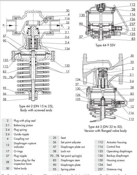
Fig. 3: Functional diagram of Type 44-2 Pressure Reducing Valve as well as Type 44-3 and Type 44-9 Safety Shut-off Valves (SSV)
