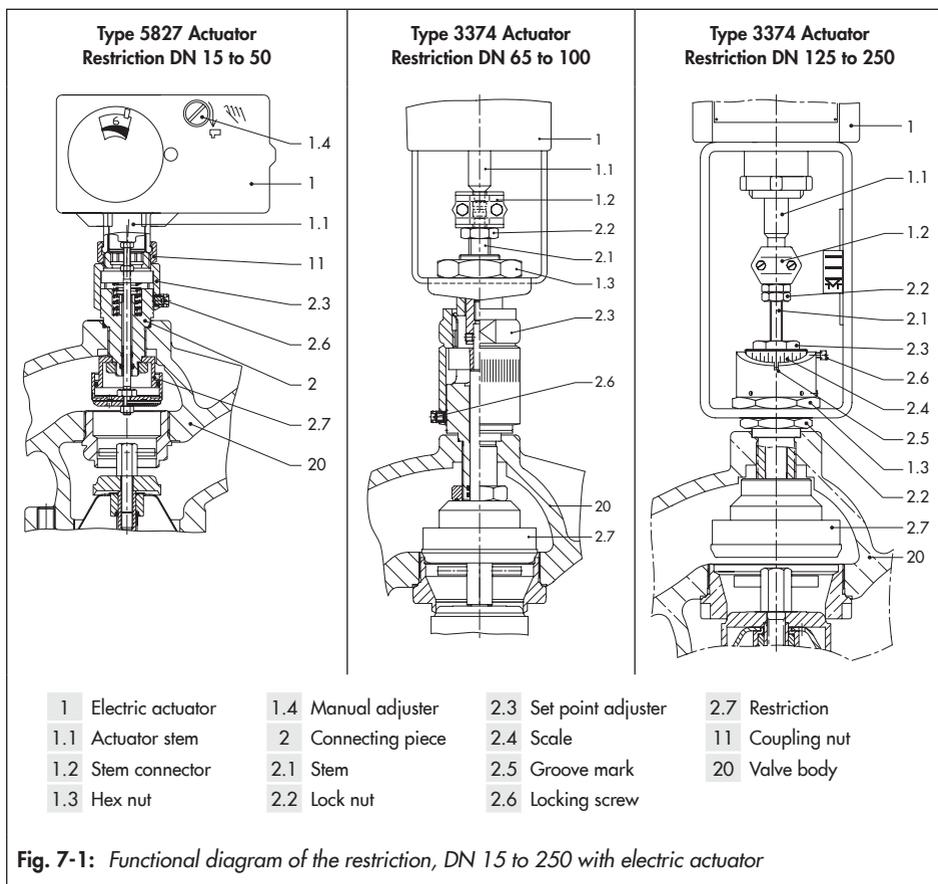
Fig. 7-1: Functional diagram of the restriction, DN 15 to 250 with electric actuator
