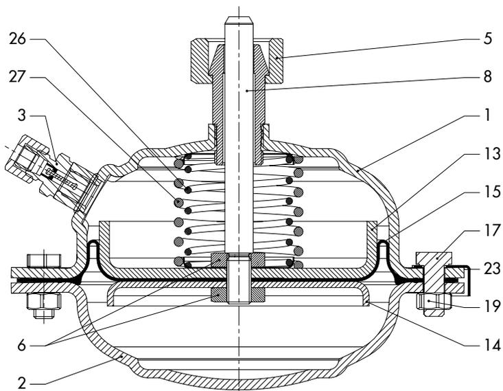
Fig. 15-5: Type 2426 Diaphragm Actuator, DN 15 to 250
