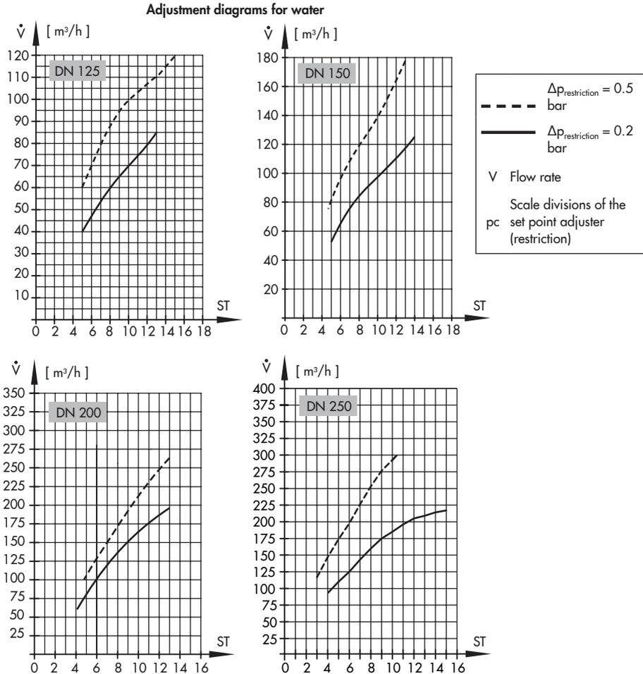
**Fig. 7-4:** Adjustment diagrams for Type 2423 E Regulator, **balanced by a bellows**, DN 125 to 250
