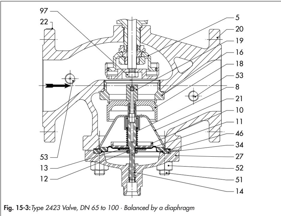
**Fig. 15-3:** Type 2423 Valve, DN 65 to 100 · Balanced by a diaphragm
