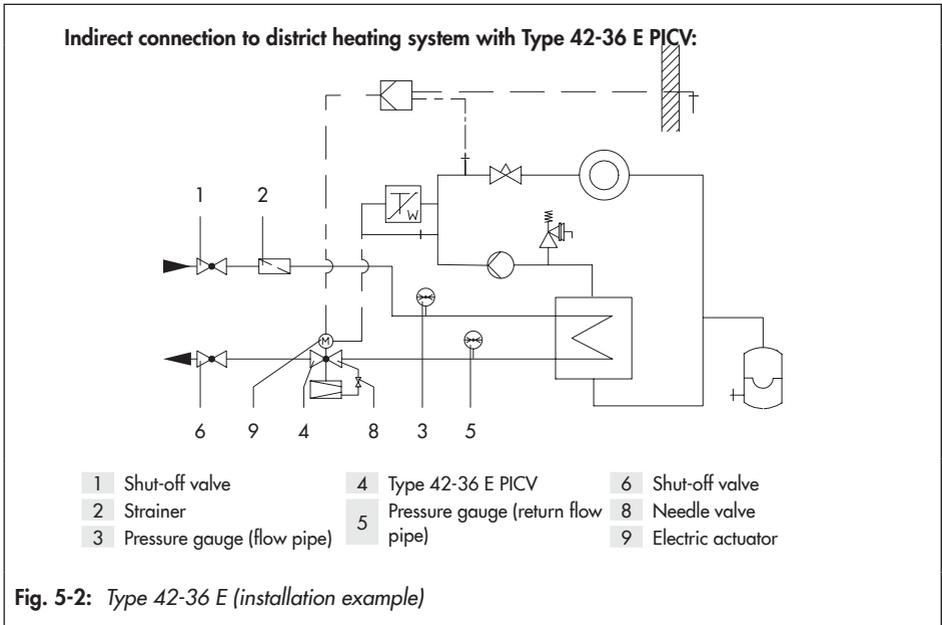
**Fig. 5-2: Type 42-36 E (installation example)**
