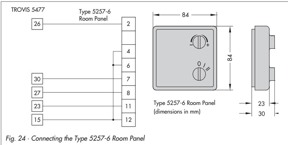
It is possible to use the room panel to correct a temperature set point or to select an operating mode when it is wired as shown above.
