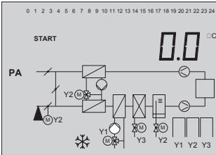
Pump ON when the outdoor temperature is smaller
