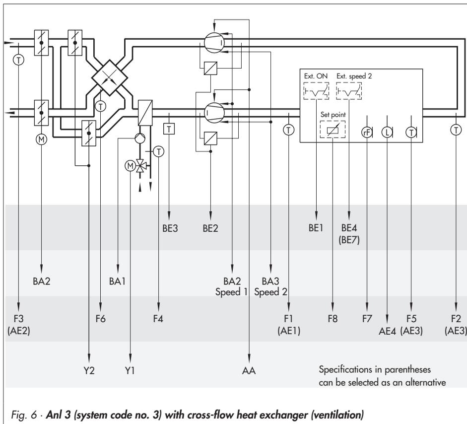
Fig. 6 · Anl 3 (system code no. 3) with cross-flow heat exchanger (ventilation)
