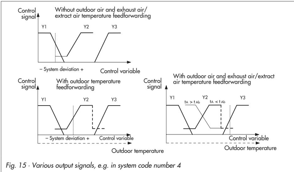
Fig. 15 · Various output signals, e.g. in system code number 4
