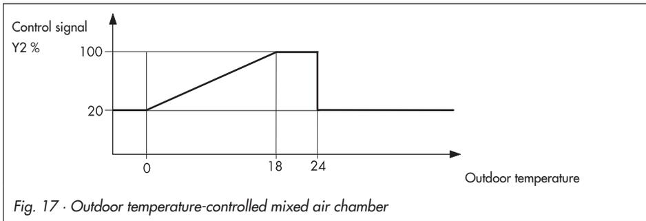
Fig. 17 · Outdoor temperature-controlled mixed air chamber
