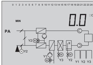
Minimum outdoor air rate when the outdoor temperature is smaller
