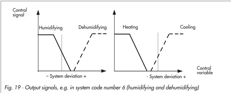
Cooling can also be controlled using an on/off signal which is issued at the binary output BA4 (→ section 6.11.7). Control of a chiller is likewise possible (→ section 6.11.8).
