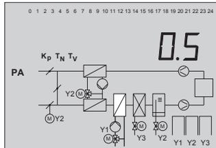
$K_p$  Heating coil (0.1 to 99.9; WE = 0,5) $T_N$  Heating coil (1 to 999 sec; WE = 60 sec) $T_V$  Heating coil (--- to 999 sec; WE = ---)
