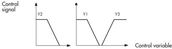
Fig. 18 · Output signals, e.g. in system code number 6 (humidifier only)
