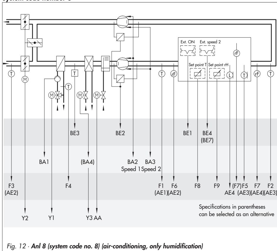
Fig. 12 · Anl 8 (system code no. 8) (air-conditioning, only humidification)
