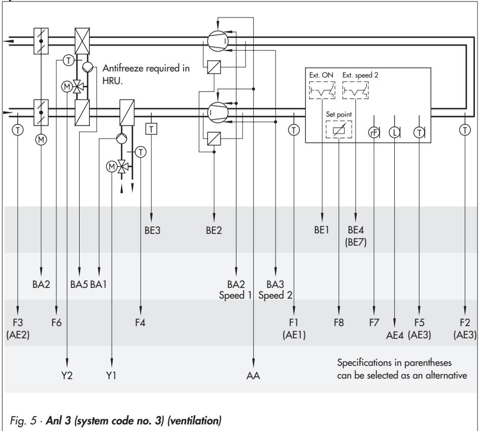
**Control of heat recovery unit (HRU) and heating coil**
