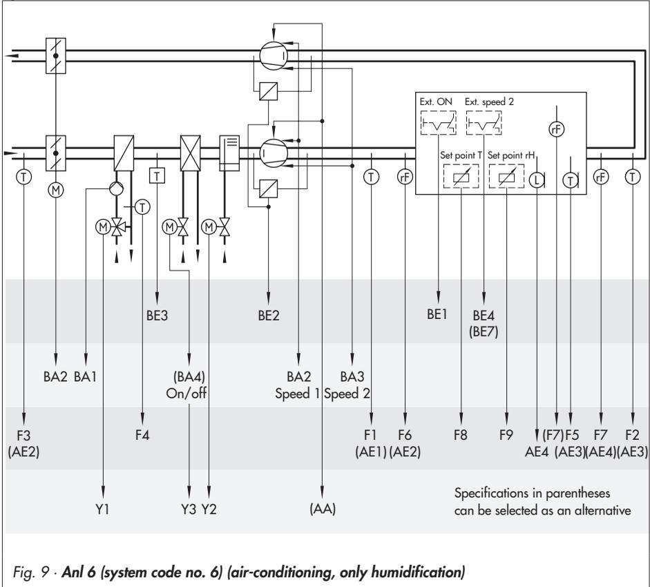
Fig. 9 · Anl 6 (system code no. 6) (air-conditioning, only humidification)
