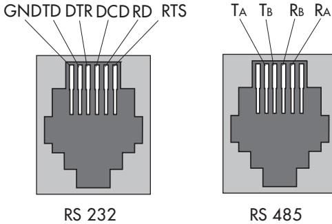
Fig. 27 · Pin assignment RS-232-C and RS-485
