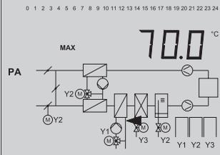
Return air temperature maximum limit (coordinate 1, 2 recognizable from the square located to the right of 1, 2)
