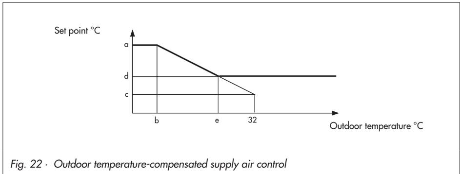
Fig. 22 · Outdoor temperature-compensated supply air control
