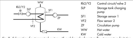
Fig. 9 · Schematics of a storage tank system with a globe valve for return flow temperature limitation
