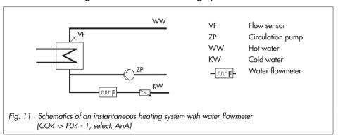
Without a flowmeter or flow switch, the required *DHW temperature* at sensor VF is only regulated during the times-of-use of the circulation pump ZP. The flowmeter or flow switch allow the controller to recognize exactly when DHW is being tapped. By deleting all the time-of-uses for the circulation pump, it is possible to regulate the required DHW temperature just while the DHW is being tapping.
