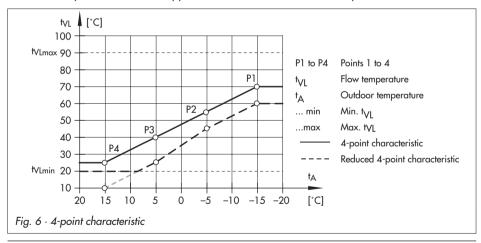
**Note:** The parameters Day set point and Night set points are no longer available when the 4-point characteristic has been selected, provided no additional functions (e.g. **Optimization**, **Flash adaptation**) have been selected.
