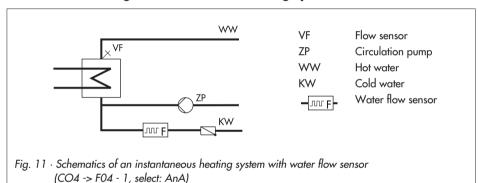
Without a water flow sensor or flow switch, the required *DHW temperature* at sensor VF is only regulated during the times-of-use of the circulation pump ZP. The water flow sensor or flow switch allow the controller to recognize exactly when DHW is being tapped. By deleting all the time-of-uses for the circulation pump, it is possible to regulate the required DHW temperature just while the DHW is being tapping.
