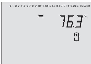
Temperatur am Speichersensoren SF2, SF3 (Pufferspeicher)
