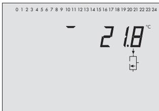
Temperatur am Speichersensor SF4 (Pufferspeicher)
