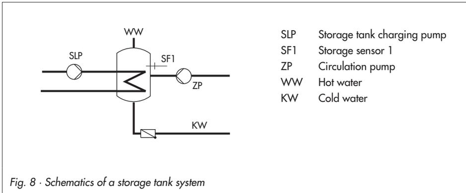
Fig. 8 · Schematics of a storage tank system
