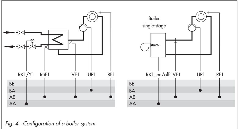
Fig. 4 · Configuration of a boiler system
