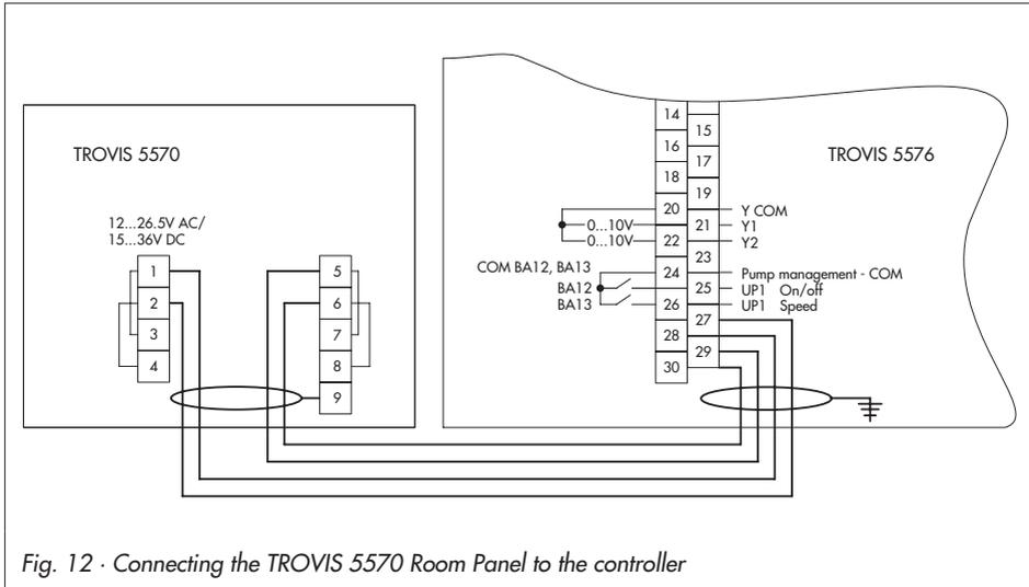
Fig. 12 · Connecting the TROVIS 5570 Room Panel to the controller
