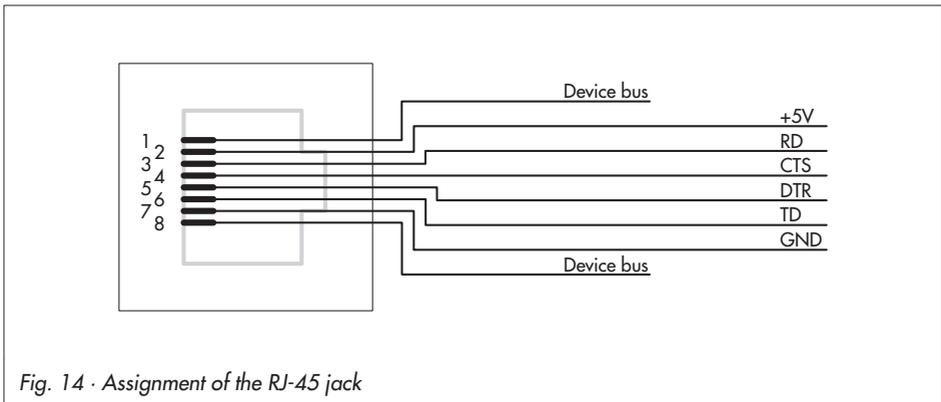
Fig. 14 · Assignment of the RJ-45 jack
