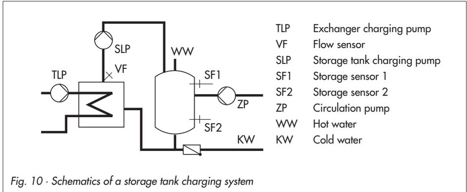
The controller begins charging the storage tank when the water temperature measured at sensor SF1 falls below the *DHW temperature set point* by 0.1 °C. If the flow temperature in the system exceeds the desired charging temperature, the controller tries to reduce the flow temperature in the heating circuit for up to 3 minutes before the exchanger charging pump is activated together with the storage tank charging pump.
