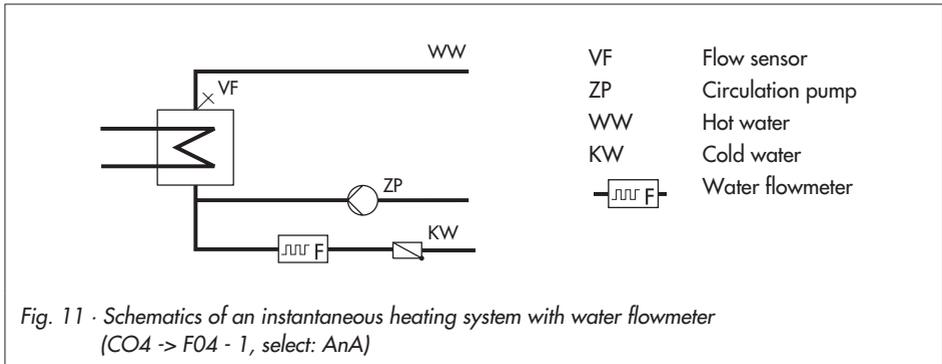
Without a flowmeter or flow switch, the required *DHW temperature* at sensor VF is only regulated during the times-of-use of the circulation pump ZP. The flowmeter or flow switch allow the controller to recognize exactly when DHW is being tapped. By deleting all the time-of-uses for the circulation pump, it is possible to regulate the required DHW temperature just while the DHW is being tapping.
