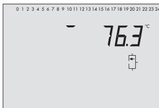
Temperatur am Speichersensoren SF2, SF3 (Pufferspeicher)
