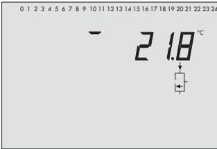
Temperatur am Speichersensor SF4 (Pufferspeicher)
