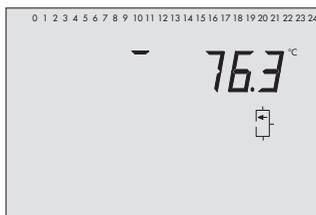
Temperatur am Speichersensoren SF2, SF3 (Pufferspeicher)
