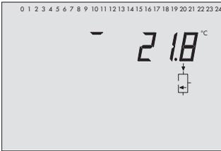
Temperatur am Speichersensor SF4 (Pufferspeicher)
