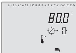
Max. charging temperature (only with VF4)
