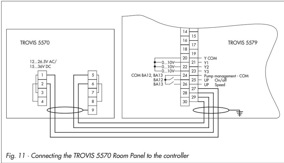
Fig. 11 · Connecting the TROVIS 5570 Room Panel to the controller
