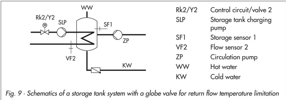
Globe valve and temperature sensor VF2 are used exclusively for return flow temperature limitation in the schematics shown above. The pre-control circuit provides at least the same flow temperature as in the standard schematic version which is calculated from *DHW temperature set point + Charging temperature boost + Boost set point of primary exchanger control*.
