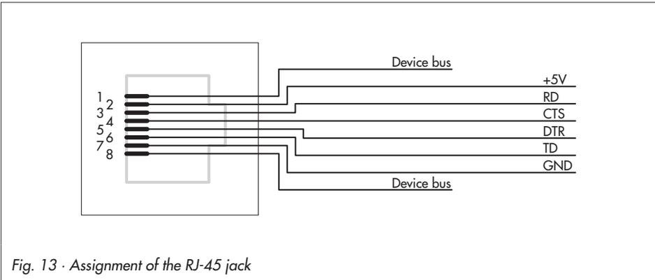
Fig. 13 · Assignment of the RJ-45 jack
