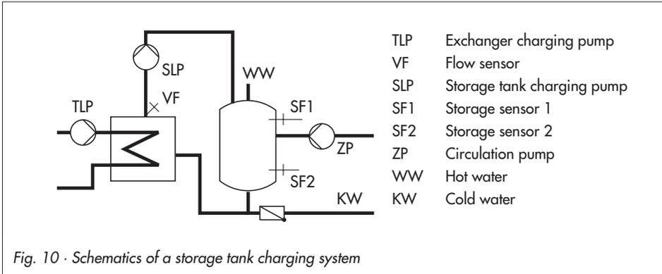
Fig. 10 · Schematics of a storage tank charging system
