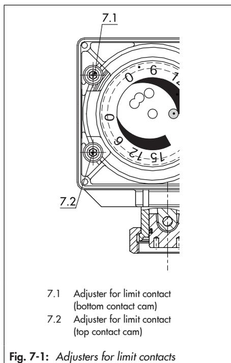
**Fig. 7-1:** Adjusters for limit contacts
