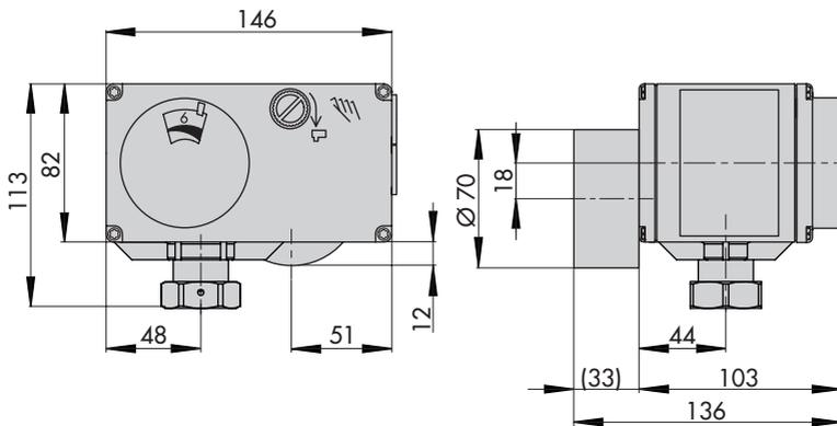
Fig. 3-2: Dimensions in mm · Types 5824/5825 (force-locking attachment)
