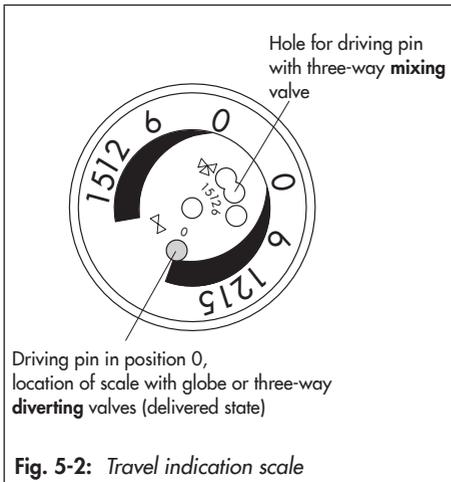
**Globe and three-way diverting valves:** the driving pin is in position 0 (delivered state).
