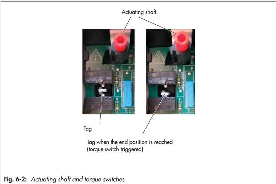
Fig. 6-2: Actuating shaft and torque switches
