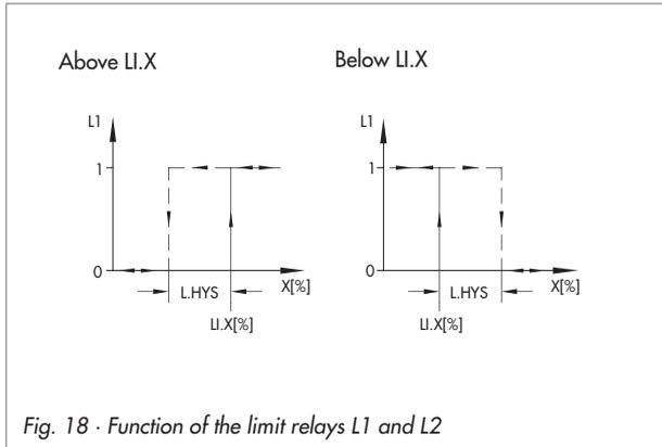
Fig. 18 · Function of the limit relays L1 and L2
