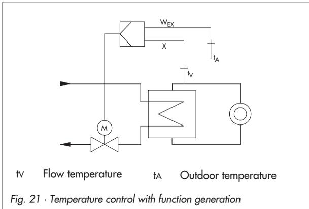
We will show you how to use function generation exemplifying an outdoor temperature-sensitive flow temperature control loop, as illustrated in Fig. 21.
