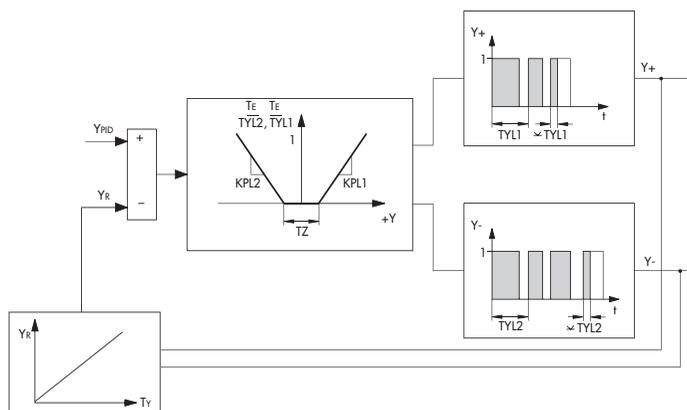
Fig. 16 · Three-step output with internal position feedback and PPM
