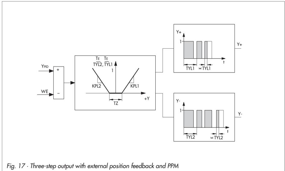
Fig. 17 · Three-step output with external position feedback and PPM
