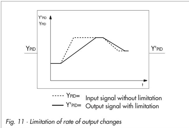
The rate of output changes can be limited for a decreasing and an increasing output variable (F03 RA.YP), for an increasing output variable (F04 RA.YP), or for a decreasing output variable (F05 RA.YP). In the limited direction(s), the output variable changes only as fast as the parameter TSRA allows it to. If the rate of output changes is slower than the defined rate of changes, limitation will not be
