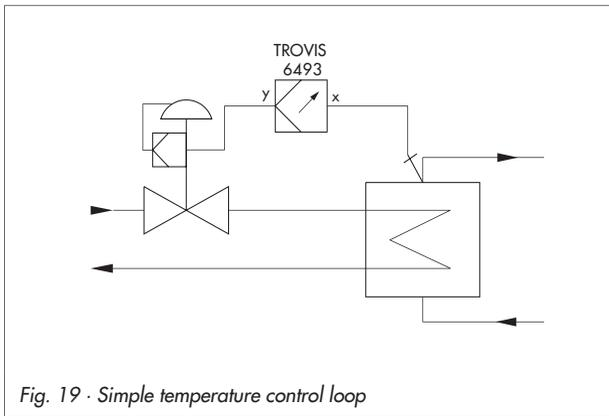
Fig. 19 · Simple temperature control loop
