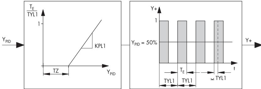
Fig. 15 · Two-step output with PPM
