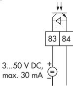
\* Note! The transmitter supply can only be used for **one** two-wire transmitter (at IN1 or at IN2) **or** for the supply of the binary input B1.
