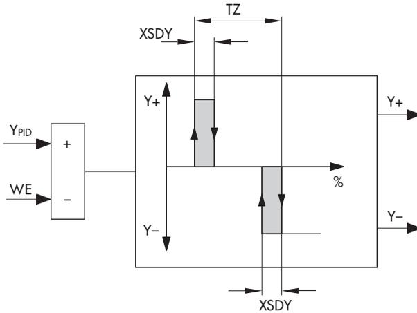
Fig. 14 · Three-step output with external position feedback
