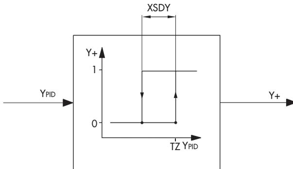
Fig. 12 · Two-step output
