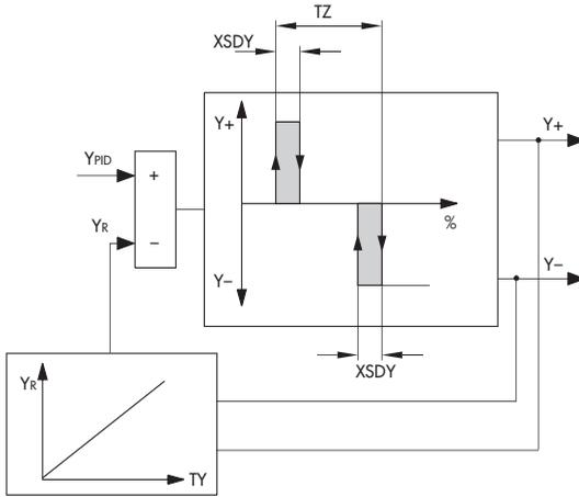
Fig. 13 · Three-step output with internal position feedback
