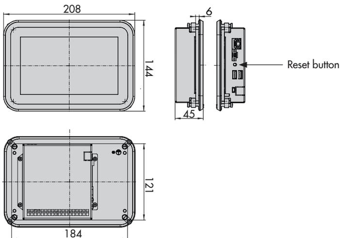
Fig. 2: Dimensions of TROVIS 6616 Web Terminal
