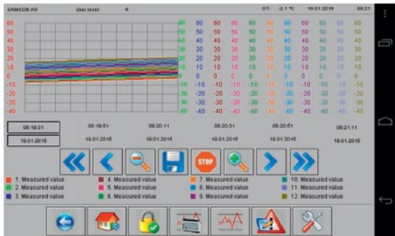
Alternatively, the automatic scaling of the Y axis can be deselected to make the graph larger.
