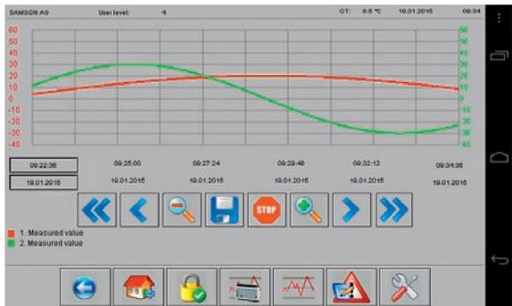
The width of the graph is reduced by the automatic scaling of the Y axis when a lot of measured data exists.
