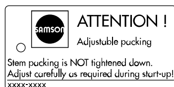
Fig. 3: Label when an adjustable packing is installed
