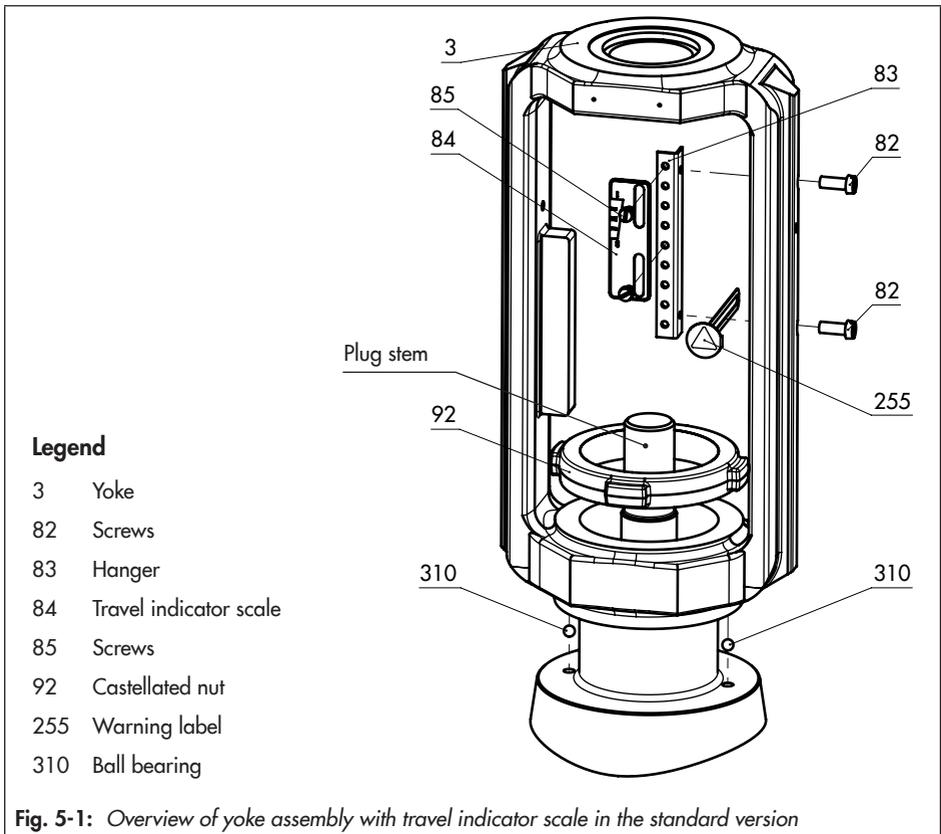
**Fig. 5-1:** Overview of yoke assembly with travel indicator scale in the standard version
