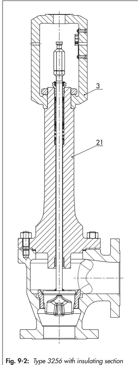
Fig. 9-2: Type 3256 with insulating section
