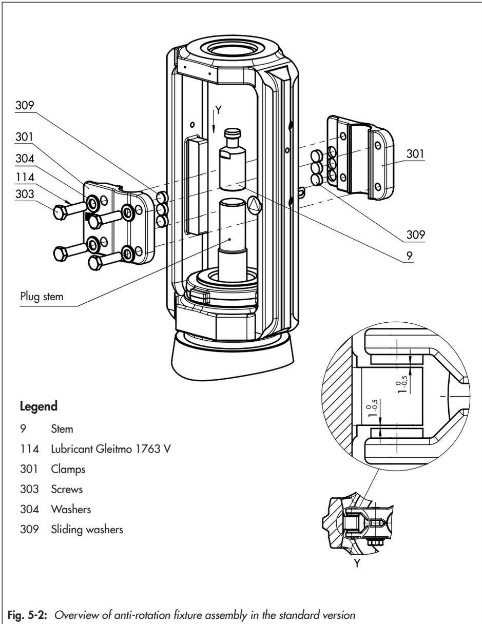
Fig. 5-2: Overview of anti-rotation fixture assembly in the standard version
