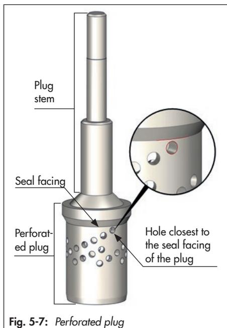
Fig. 5-7: Perforated plug
