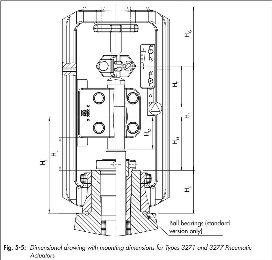
**Fig. 5-5:** Dimensional drawing with mounting dimensions for Types 3271 and 3277 Pneumatic Actuators
