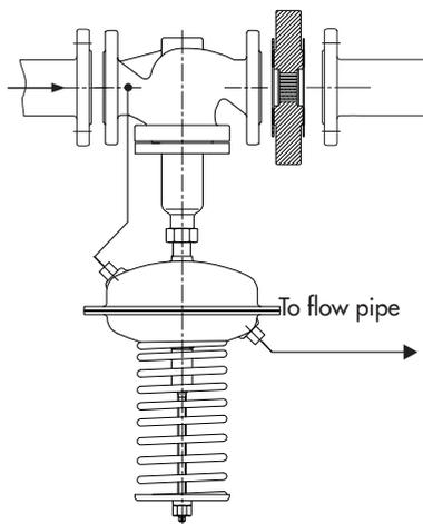
Fig. 5-4: Differential pressure regulator (closing) in the return flow pipe
