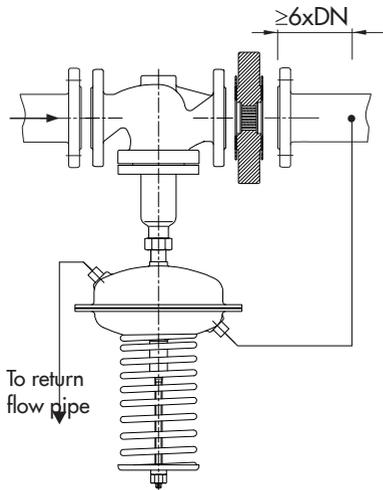
Fig. 5-3: Differential pressure regulator (closing) in the flow pipe
