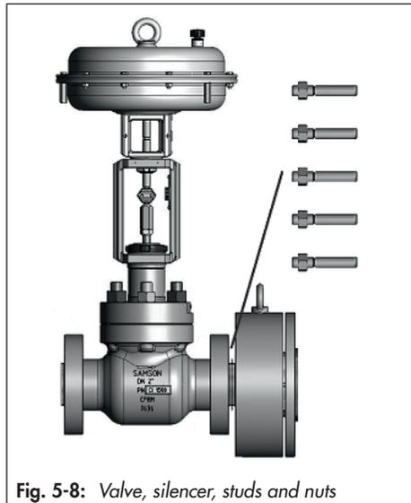
**Fig. 5-8:** Valve, silencer, studs and nuts
