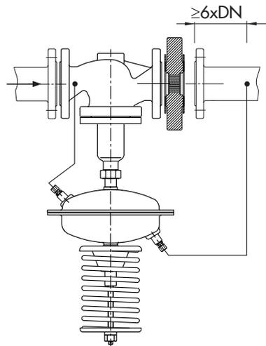
Fig. 5-2: Differential pressure regulator (opening)
