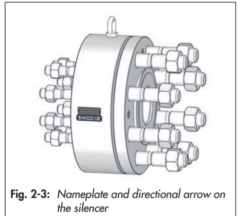
Fig. 2-3: Nameplate and directional arrow on the silencer
