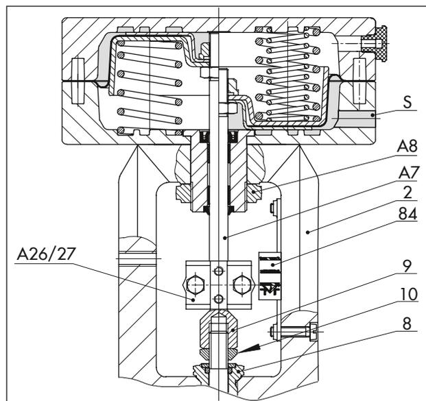
**Fig. 20:** Type 3271 Pneumatic Actuator on a Series 240 Valve
