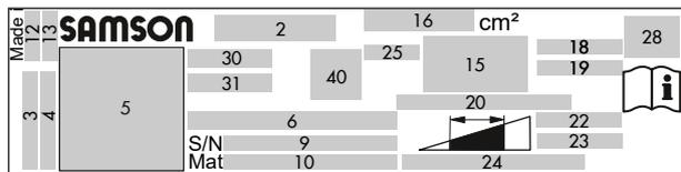
**Fig. 1:** Inscriptions on the nameplate of Type 3271/3277 or Type 2780 Actuators with 120 cm<sup>2</sup> actuator area
