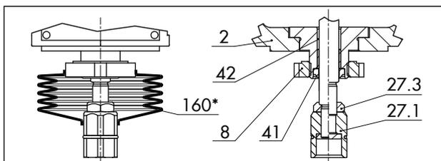
Fig. 24: Connection to version for micro-flow valve
