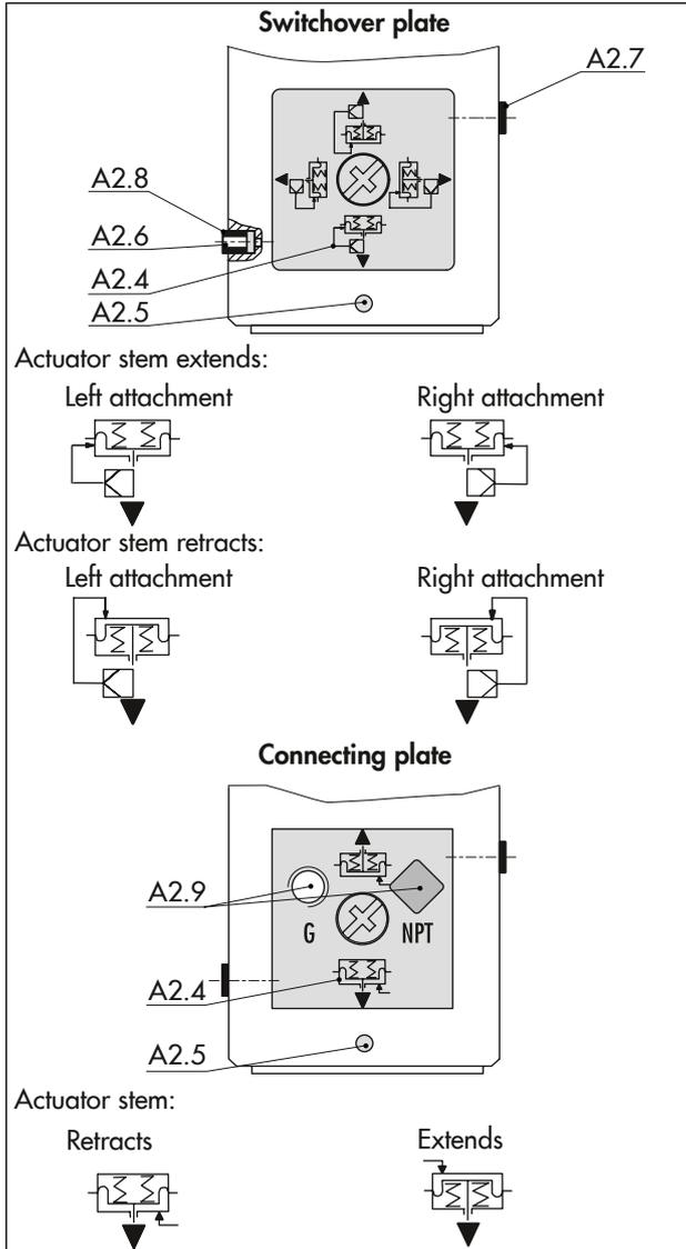
Fig. 6: Switchover plate and connecting plate on Type 3277-5
