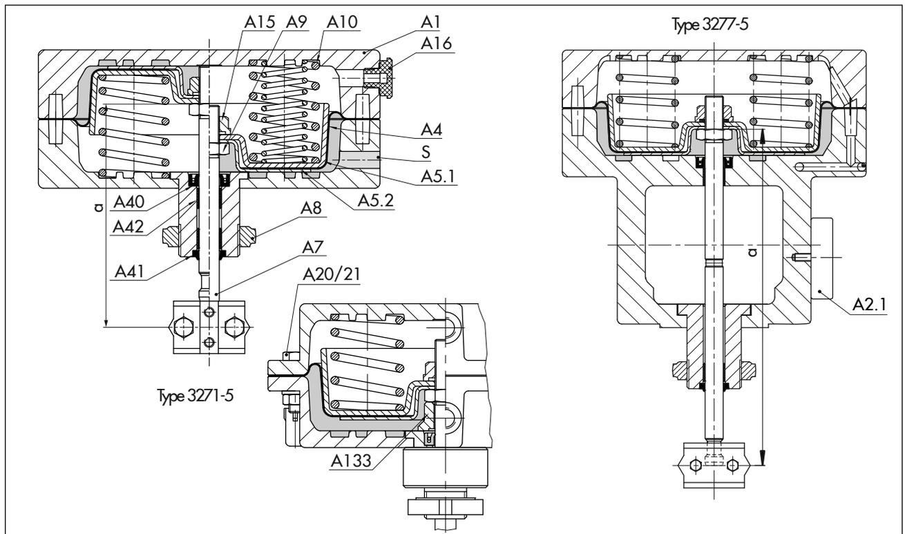
**Fig. 18:** Type 3271-5 and Type 3277-5 Pneumatic Actuators
