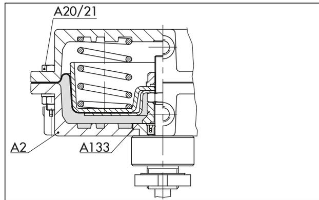
**Fig. 3:** Type 3271-5 Actuator (actuator stem extends)
