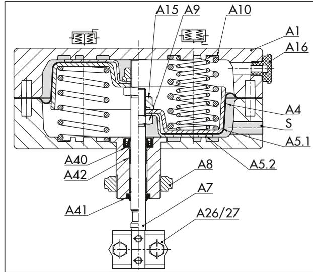
**Fig. 2:** Type 3271-5 Actuator, drawing showing an example with 120 cm<sup>2</sup> actuator area
