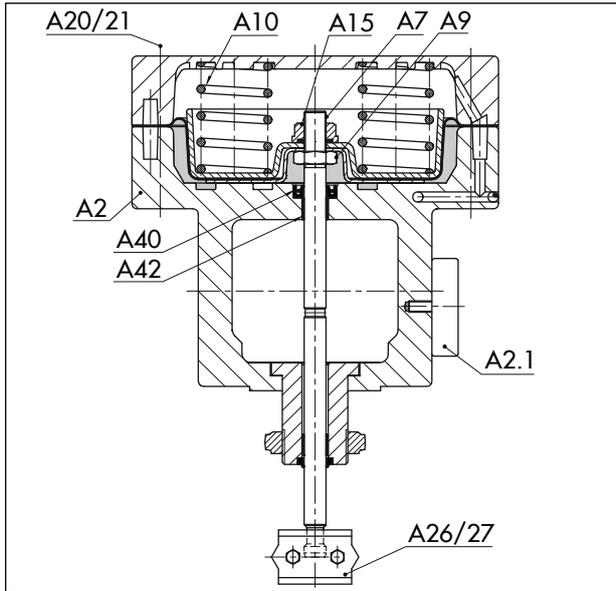
**Fig. 4:** Type 3277-5 Actuator with 120 cm<sup>2</sup> actuator area
