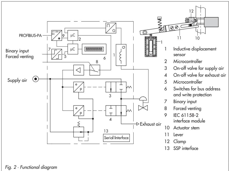
Fig. 2 · Functional diagram
