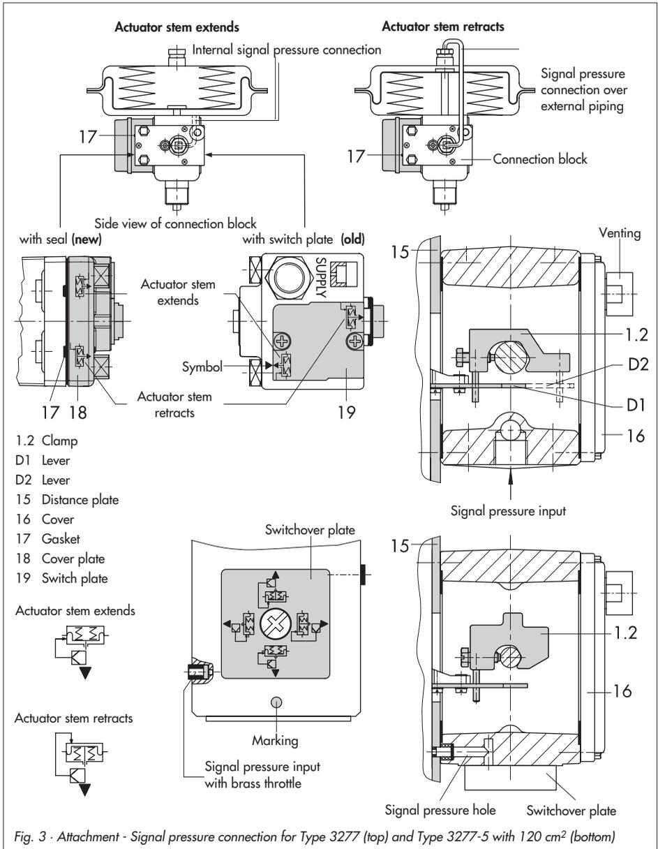
Fig. 3 - Attachment - Signal pressure connection for Type 3277 (top) and Type 3277-5 with 120 cm<sup>2</sup> (bottom)
