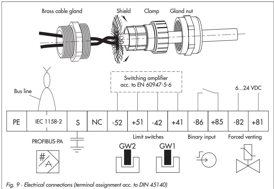
Fig. 9 · Electrical connections (terminal assignment acc. to DIN 45140)
