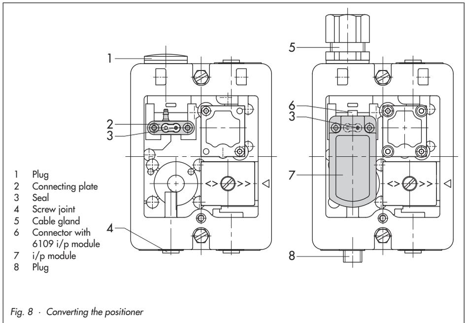
7. Fasten i/p module in the housing using the two screws. Make sure that the seal (3) with the restriction is properly positioned in the module. The restriction must be located over the right bore hole of the housing (looking from above), see Fig. 8.
