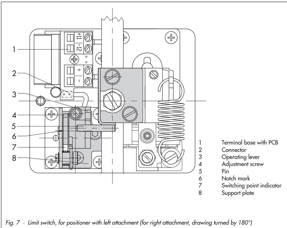
Fig. 7 · Limit switch, for positioner with left attachment (for right attachment, drawing turned by 180°)
