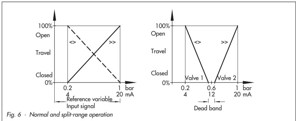
The starting point (zero) in this case is 0.2 bar or 4 mA, the upper range value is 1 bar or 20 mA.
