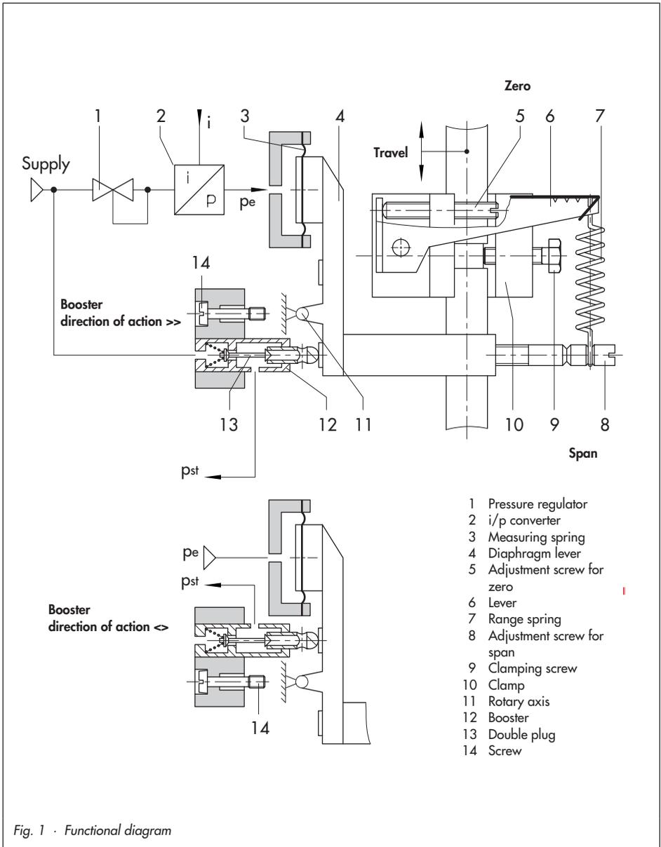
Fig. 1 · Functional diagram
