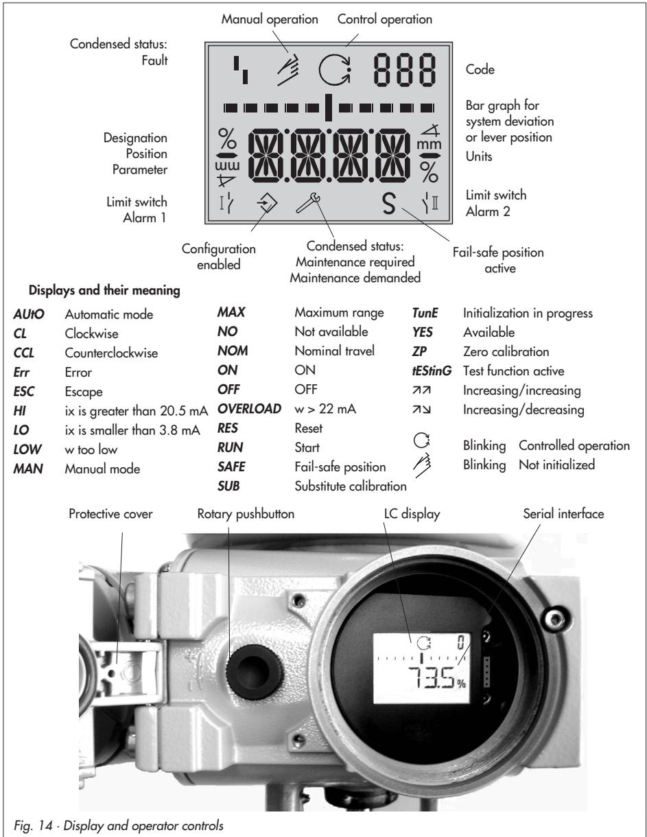
Fig. 14 · Display and operator controls
