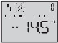
After setting the fail-safe position, it is sufficient for standard operation to start the initialization procedure (section 5.5 on page 39) in order to ensure optimum positioner operation.
