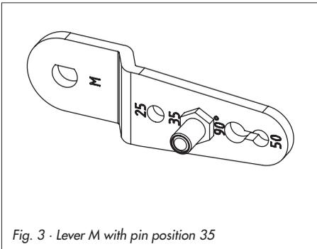
Fig. 3 · Lever M with pin position 35
