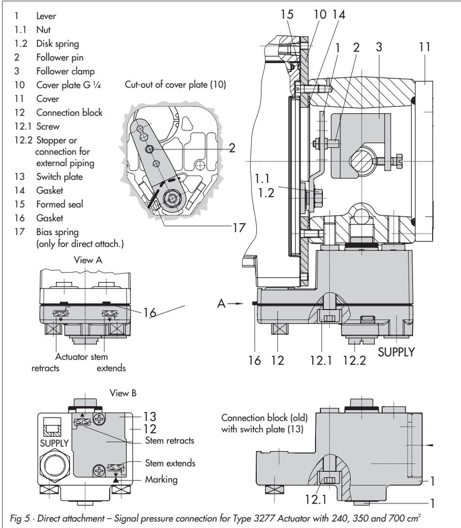
plate (13) to be turned such that the corresponding actuator symbol points to the marking.
