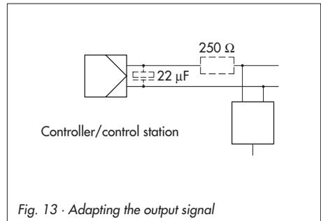
Fig. 13 · Adapting the output signal
