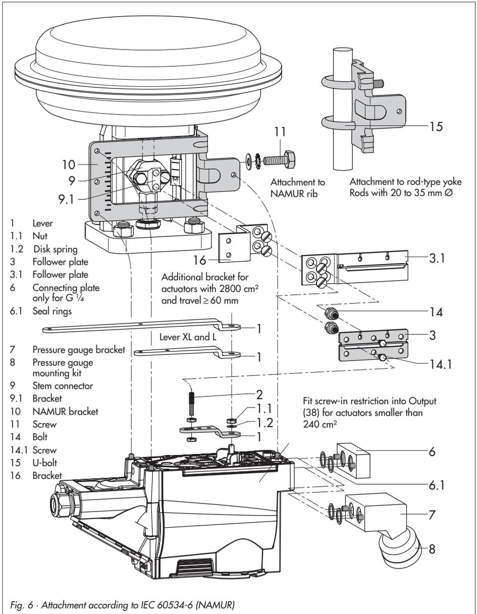
6. Place lever (1) on the positioner shaft and screw tight using the disk spring (1.2) and nut (1.1).
