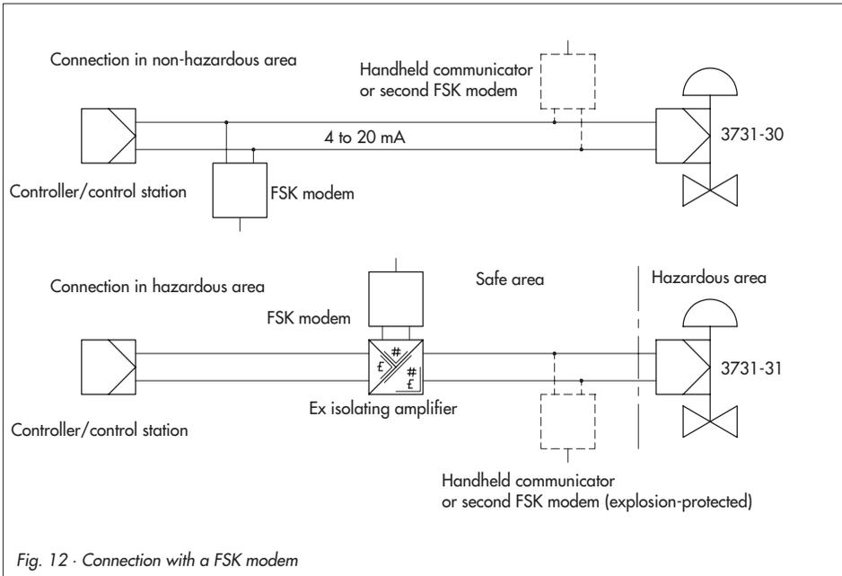
Fig. 12 · Connection with a FSK modem
