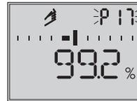
If the positioner has not yet been initialized, the position of the pick-up rod is indicated in the operating range of  $\pm 10$  mm.
