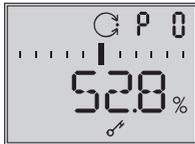
*Initialization successfully completed, positioner runs in closed-loop operation*
