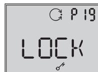
***LOCK** and the key icon indicate that the configuration is locked.*
