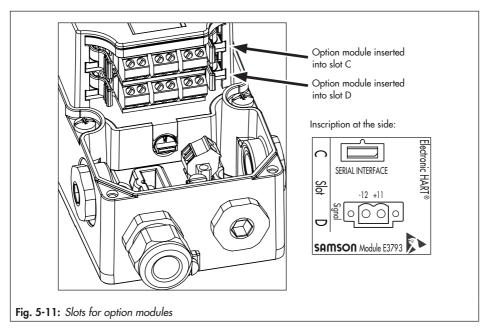
When option modules are used, either two option modules or an option module and a dummy module must be installed. A slot without an installed module is not permissible
