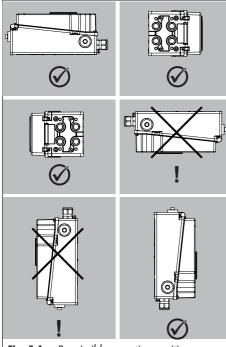
Fig. 5-1: Permissible mounting positions
