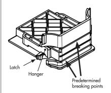
Dummy module in the delivered state
