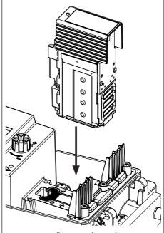
**Fig. 5-6:** Installing or replacing the pneumatic module
