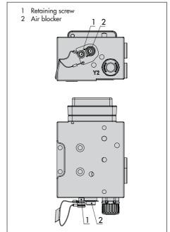
Fig. 5-23: Adapter block for attachment according to VDI/VDE 3847-2
