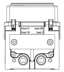
Fig. 5-33: Output 238 and Exhaust 79 sealed with dummy plate
