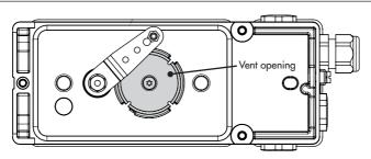
Fig. 5-2: Vent opening (back of the positioner)
