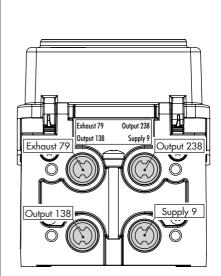
Fig. 5-32: Pneumatic outputs
