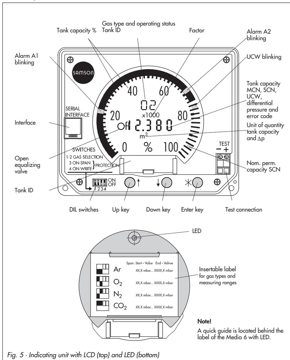
Fig. 5 · Indicating unit with LCD (top) and LED (bottom)
