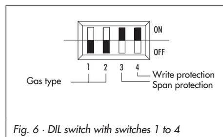
Fig. 6 · DIL switch with switches 1 to 4
