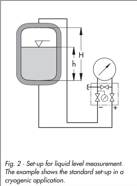
Fig. 2 · Set-up for liquid level measurement. The example shows the standard set-up in a cryogenic application.
