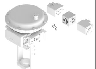
Redundancy block: emergency venting, extended NAMUR interface ¼ – 1oo2
