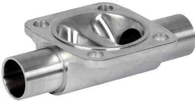
Through the forging procedure a high density and homogeneous structure of the material is generated. This reduces the possibility of porosity or that any inclusions can emerge. After that, the forged body is mechanically machined according to specifications.
