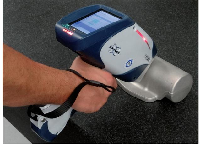
Spectrometer and XRF spectroscopy material analysis
