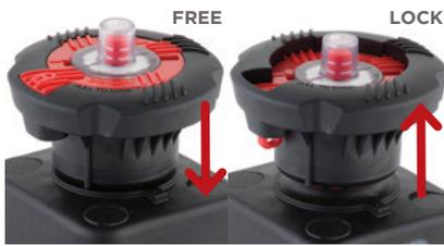
The 882 valve is equipped with a handwheel locking system that prevents the valve from being operated. The system can be engaged by simply lifting the handwheel once the required position has been reached (fig. 8). To release the operating mechanism, simply return the handwheel to its previous position by pushing it downwards (fig. 6). When the system is in the locked position, a lock can be installed to protect the plant against unwanted interference (fig. 9).
