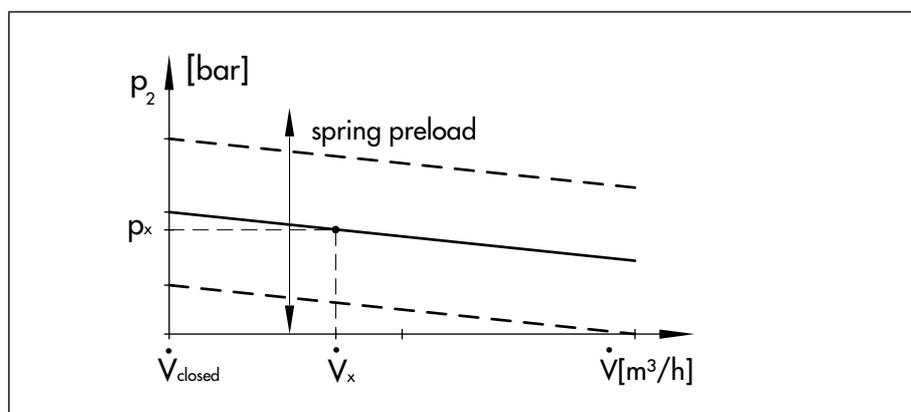
Fig. 7: Ideal characteristic of a pressure reducing valve
