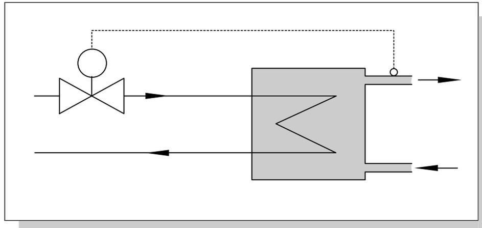
Fig. 2: Control loop with self-operated regulator
