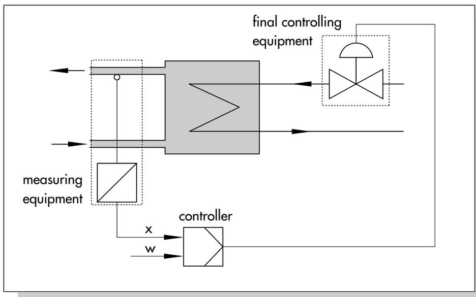
Fig. 1: Control loop with conventional instrumentation
