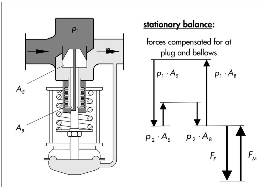
Fig. 8: Balance of forces in a pressure reducing valve with plug balanced by a bellows
