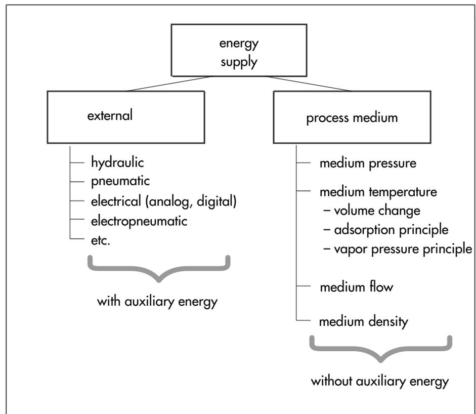
Fig. 3: Energy supply of control equipment
