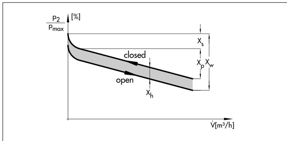
Fig. 9: Characteristic of a pressure reducing valve
