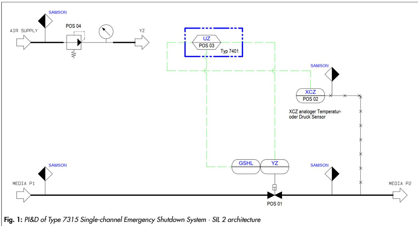
Fig. 1: PI&D of Type 7315 Single-channel Emergency Shutdown System - SIL 2 architecture
