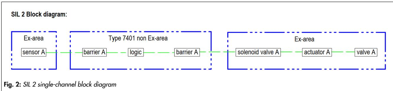
Fig. 2: SIL 2 single-channel block diagram
