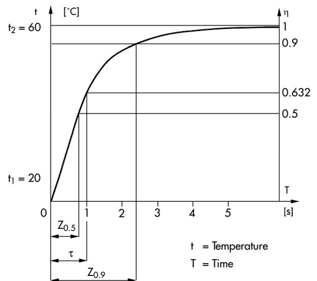
Fig. 2 · Transfer function of the Type 5209 Sensor
