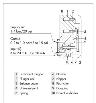
Fig. 2: Functional diagram of Type 6112-02 i/p Converter Module
