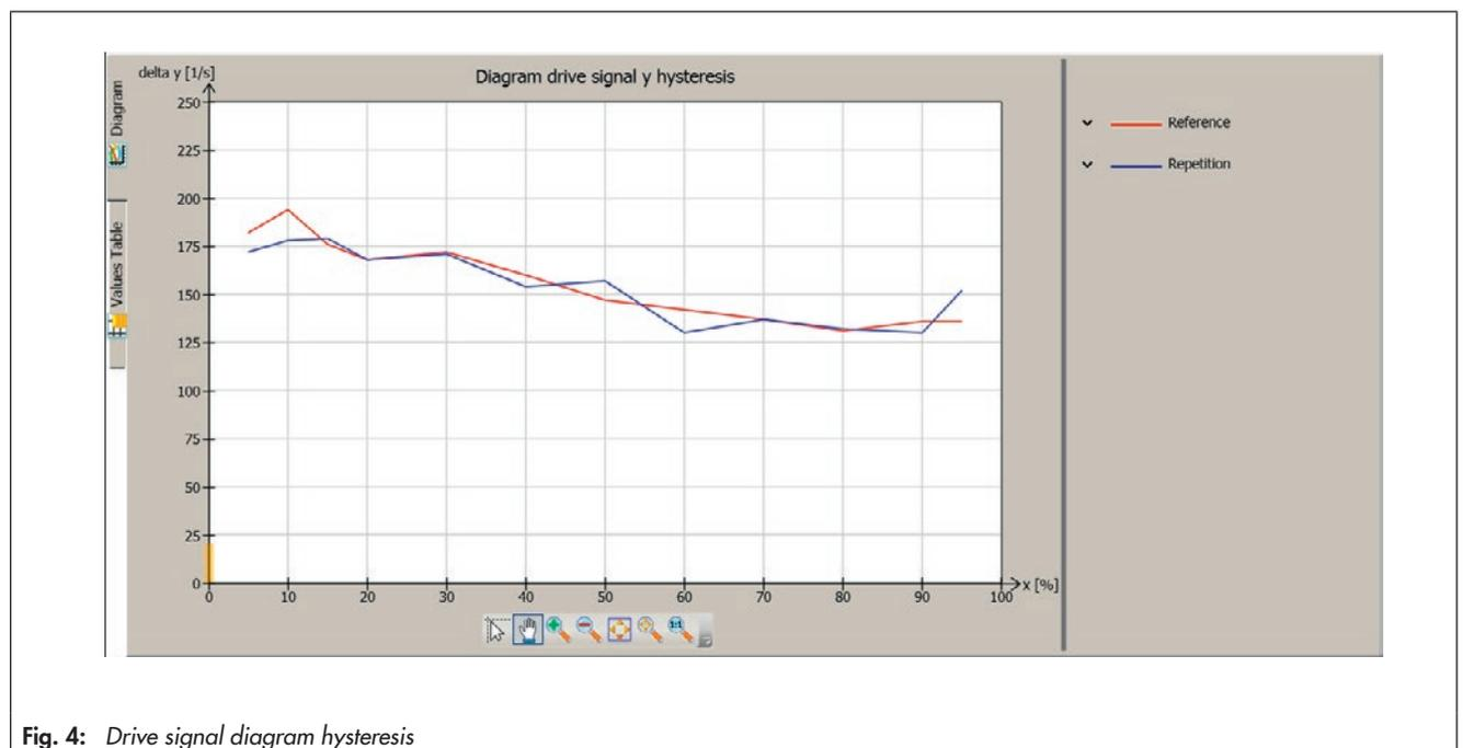
Fig. 4: Drive signal diagram hysteresis
