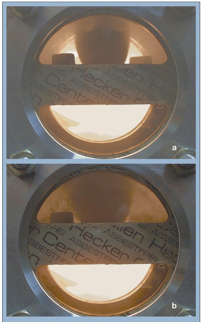
**Fig. 3.** Visualization of cavitation (a) and flashing (b) with flow coming from below.
