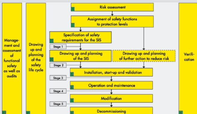
Fig. 2: Safety life cycle according to IEC 61511-1, Fig. 8
