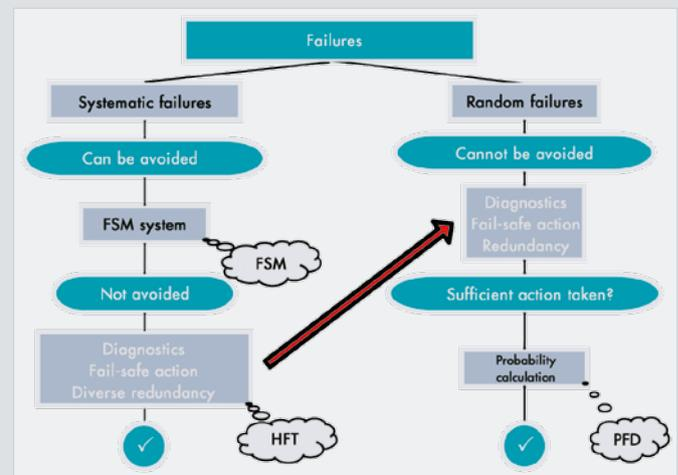
Fig. 1: Causes of failure according to [4]
