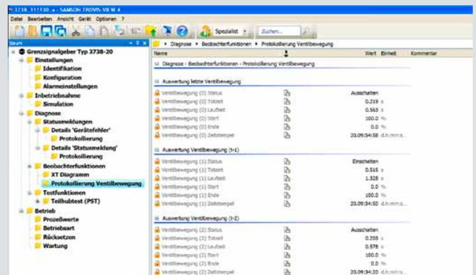
Fig. 4: Logging of valve movements
