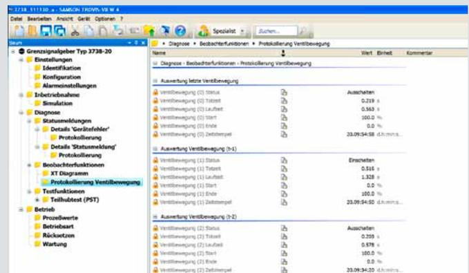
Fig. 4: Logging of valve movements
