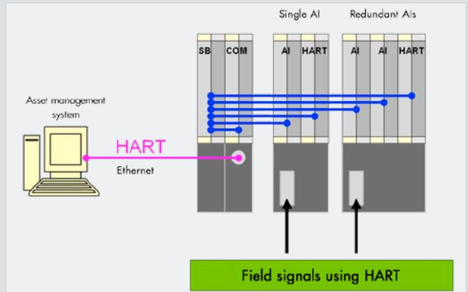
Fig. 7: Tunneling of HART® signals
