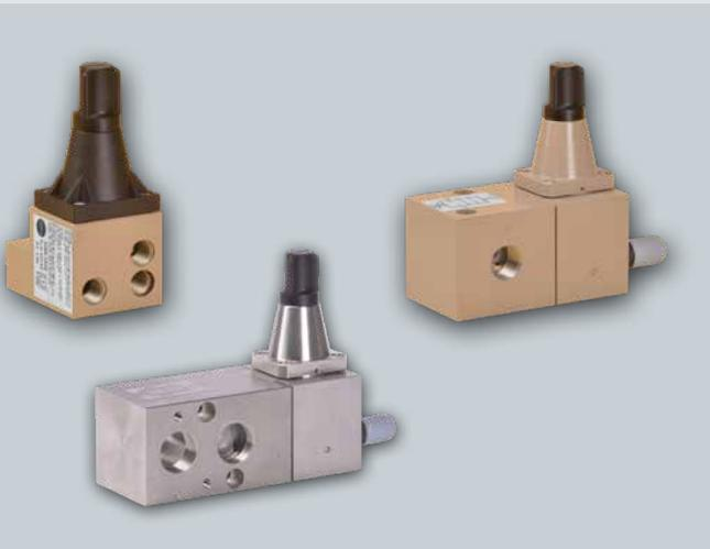
Lock-up valves are used to shut off the signal pressure line of pneumatic actuators. They shut off the line either when the air supply falls below an adjusted limit or in case of complete air supply failure. This causes the actuator to fail in place.
