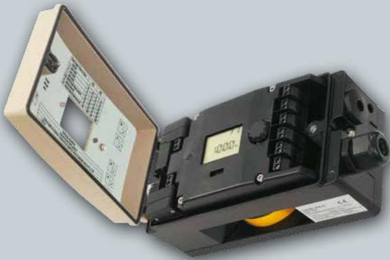
Limit switches are suitable for automation of on/off applications and issue an electric binary signal when the valve travel exceeds or falls below an adjusted limit. The signal can be used, for example for switching control signals, issuing visual and audible alarms or for connection to central control or alarm systems.
