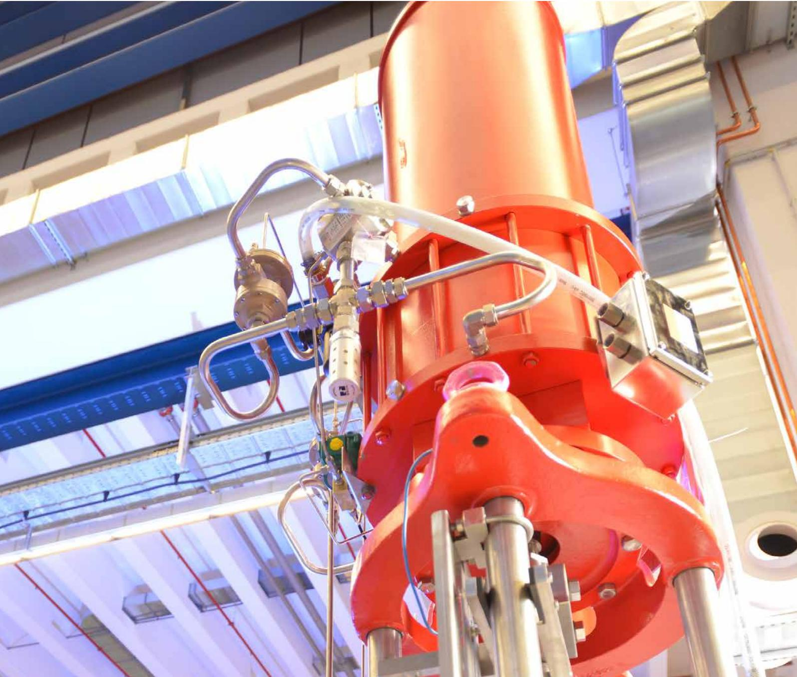
Limit Switches · Solenoid Valves
