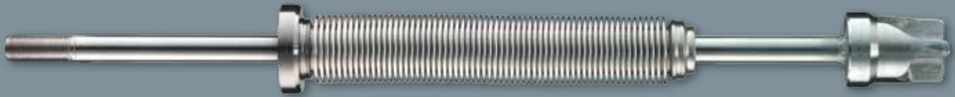
Metal bellows are used in globe valves to seal the plug stem to the atmosphere. The thin-walled corrugated cylinders are used as dynamic seals, particularly in applications where strict emission requirements apply. Metal bellows by SAMSON are made of corrosion-resistant materials. They are capable of withstanding high pressures and temperatures, which makes them ideally suited for use in high-performance service.
