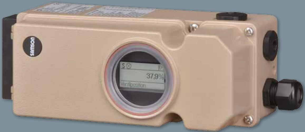
The EXPERTplus valve diagnostics integrated into the positioner provide reliable information on the condition of the metal bellows. The measured data are assessed based on a statistical analysis of the cycle heights that the valve moved through. The positioner issues a classified status message in compliance with NAMUR Recommendation NE 107 when a critical condition exists.
