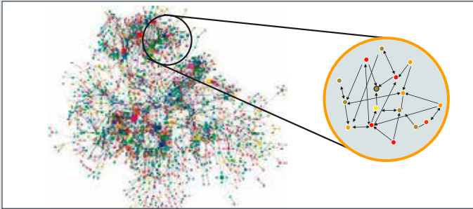
Fig. 3: The software represents the plant as a mathematical graph that contains the relations between the different components.
