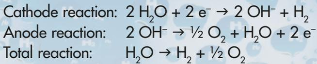
Benefits of alkaline electrolysis include a long durability and high plant performance. Based on the operating principle, water is introduced at the cathode using the alkaline electrolyte circuit.
