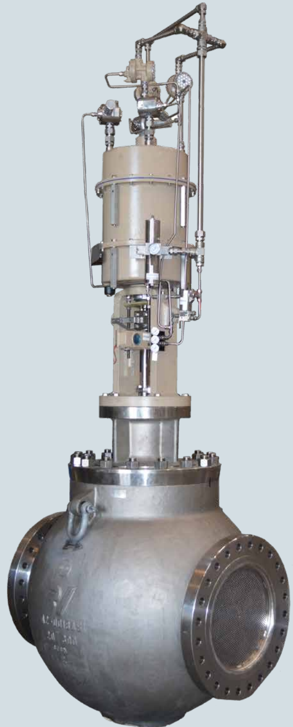
Fig. 7: 20" anti-surge valve with pneumatic actuator and control system to ensure fast acting via solenoid (emergency condition) and via positioner (control)
