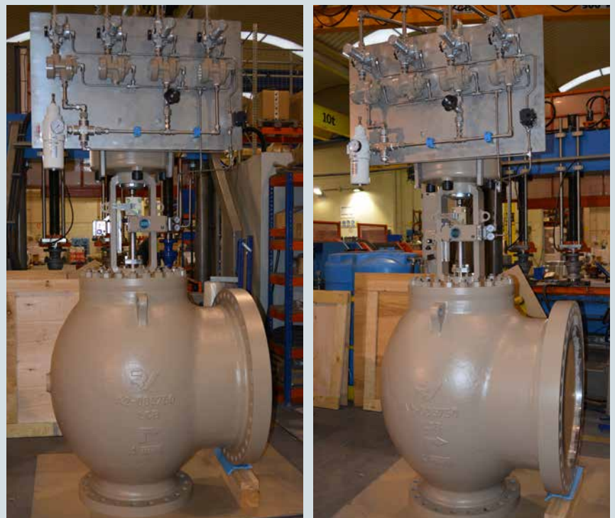
Fig. 6: Type 3595 Valve with an asymmetric angle body for anti-surge service in an ethane compressor
